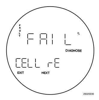
Figure 6-11. Fault 7, Reversed O<sub>2</sub> Cell
